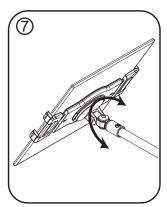
The tablet can tilt up and down by 180°.
