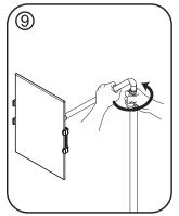
Loosen the knob to adjust the height and the angle of the tablet.
