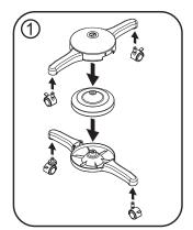
Assemble the base and then insert casters into the bottom of the base.
