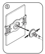
Attach the tablet holder to the top of the pole.
