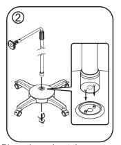
Place the pole at the center of the base and insert the screw from the bottom and tighten it.
